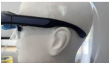
Virtual Reality Device Comfort Test
