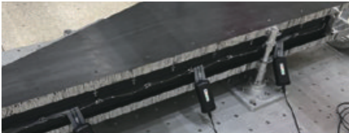
Sector solar cell wing binding test
