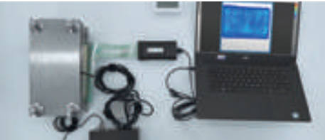
Charge/discharge stress test for battery cell module
